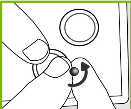
**2** Push pin to button bottom and rotate ~ 45° towards button cap.
