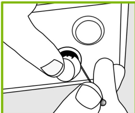
**3** Place finger over cap, pull up on pin to lift cap out of the box.
