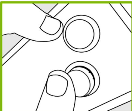
**4** Insert new cap into button hole and rotate until cap is in place.
