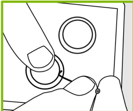
**1** Insert removal pin between button cap and outer button ring.
